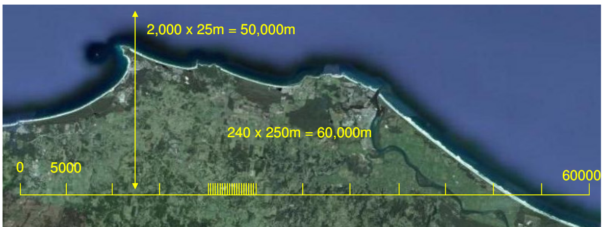
Figure 8: Model extent and grid element representation
